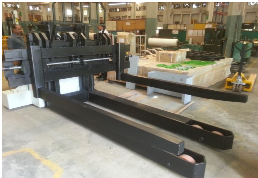
Fig10: Finished stacker with complete assembly and painting
